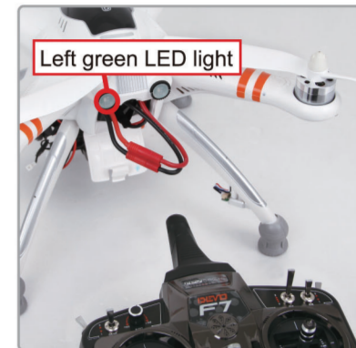
6.6 The left green LED flash quickly till light out which means calibration finished. Please reconnect the aircraft power after calibration.
