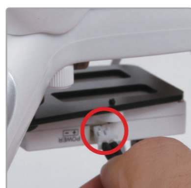
4.3 Plug the camera cable into the gimble controller.
