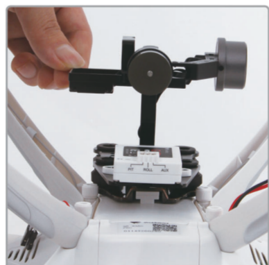
3.3 Done, the gimble is installed.
