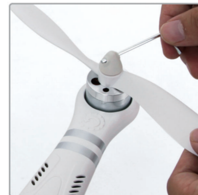
2.3 Screw the "spinner" on. Then tighten using one of the allen wrenches in the kit.
