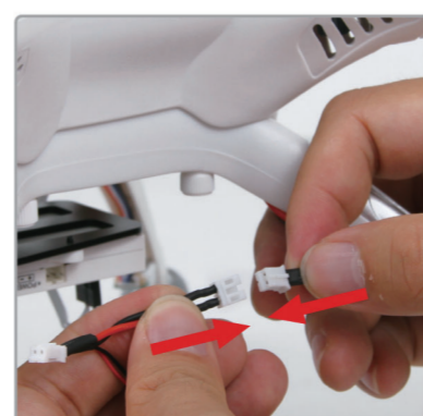
4.4 Connect the camera cable to the power wire from the QR X350PRO quad.
