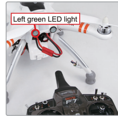
5.4 When the LEFT indicator light stop flashing, the binding is successful.
