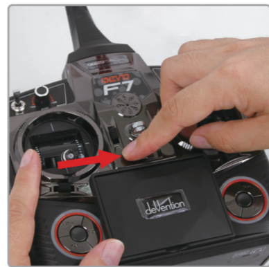
5.2 Move the MIX and FMOD switches to "0" position. Move the throttle to the down position. Then turn on the radio.
