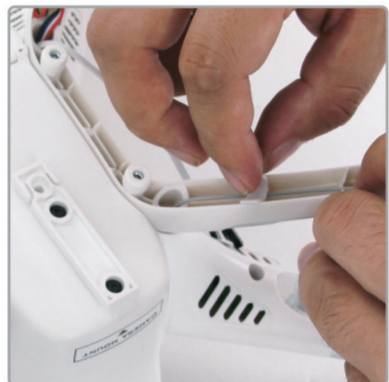
1.8 Secure the cable into the hollow part of the leg with one of the supplied foam tape strips.
