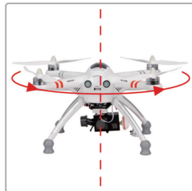
6.4 Horizon level 360° rotation (Rotate the aircraft, from 0° to 90°, 180°, 270°, 360°, all need to pause for 1 second.)
