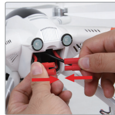
5.3 Connect the battery to the quad. Before powering the quad, make sure the quad is level and sitting stable on the ground, do not move the quad until the binding is finished.
