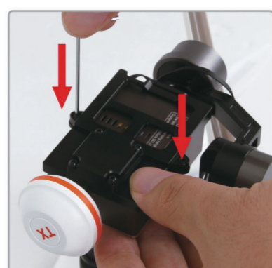
4.2 Secure the camera with the mounting bracket, the bracket have a rounded cut for the lens.
