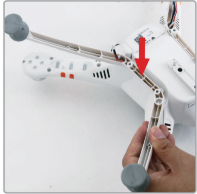
1.4 Install the left skid, carefully pull the cable through the hole in the landing gear.
