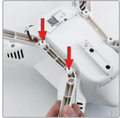
1.5 Secure the landing gear with 2 screws, tighten firmly with your fingers, do not use tools.
