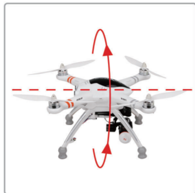
6.3 Leftward & rightward 360° rotation (Rotate the aircraft, from 0° to 90°, 180°, 270°, 360°, all need to pause for 1 second.)
