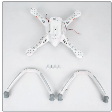
1.1 Prepare quadcopter landing gear and 4 screws.
